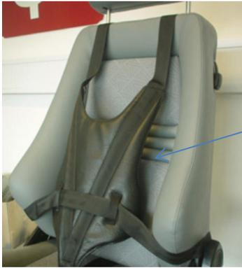
The person is now fixed in the seat. Make sure the belt is closed and adjusted.
