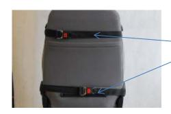
Place the 2 horizontal straps attached to the vest around the backrest, set and lock them.
